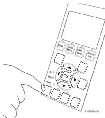
Figure 4. 51: Step 5: After pressing the [Hand on] button, the LED above the button should be lit and the motor may rotate.
