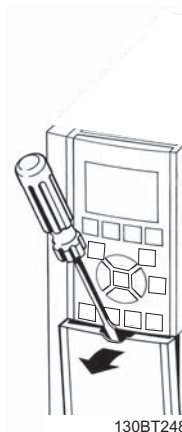
Figure 4.44: Access to control terminals for A2, A3, B3, B4, C3 and C4 enclosures
